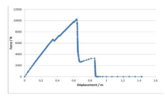
Fig. 3. Root anchorage response curve with *Pinus pinaster* root properties taken from Dupouy (1992): Young's modulus: 1-1.2GPa; tensile strength: 40MPa; compressive strength: 35MPa
