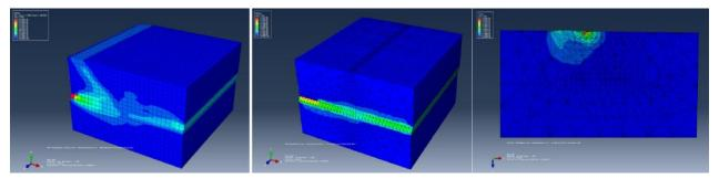
Fig 1. Distribution of equivalent plastic strain during a simulation of reinforced soil shear test using embedded beam elements (a), solid elements with frictional behaviour (b). Plastic strains during a tree overturning (c).
