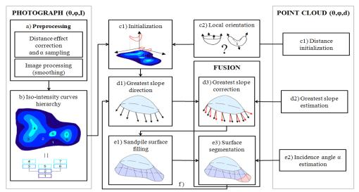
Fig 1. Algorithm flowchart for the surface reconstruction.
