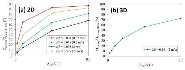
Fig. 2. Surface-averaged convective scalar flows at the leaf surface as a function of the coverage ratio, for CR up to 10%. The flows are scaled with the surface-averaged scalar flow for a coverage ratio of 100%  $(Q_{c,w,avg,100\%})$ : (a) 2D model at different air speeds  $(U_b, i.e., d/\delta_{VSL})$  ratios); (b) 3D model at a single air speed.
