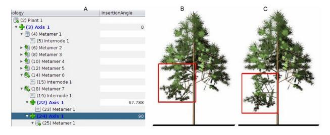
Fig. 1. Editing in the Xplo table view: (A) changing the insertion angle of the selected branch (B) of a juvenile Black pine tree is directly shown in the 3D view (C) when the on-the-fly geometric reconstruction is activated.
