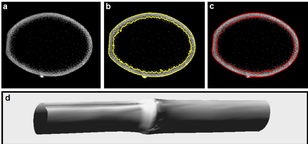
**Figure 3:** Representative corn stalk cross-sections: (a) axial CT image (179KB); (b) image overlaid with edges detected by level-set method (edges require 16KB); (c) smoothed & simplified edges contours (requiring less than 1KB total); (d) digitized surface model (15KB for shown geometry).
