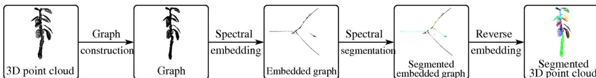
Fig. 1. Pipeline of the segmentation method proposed in this study.
