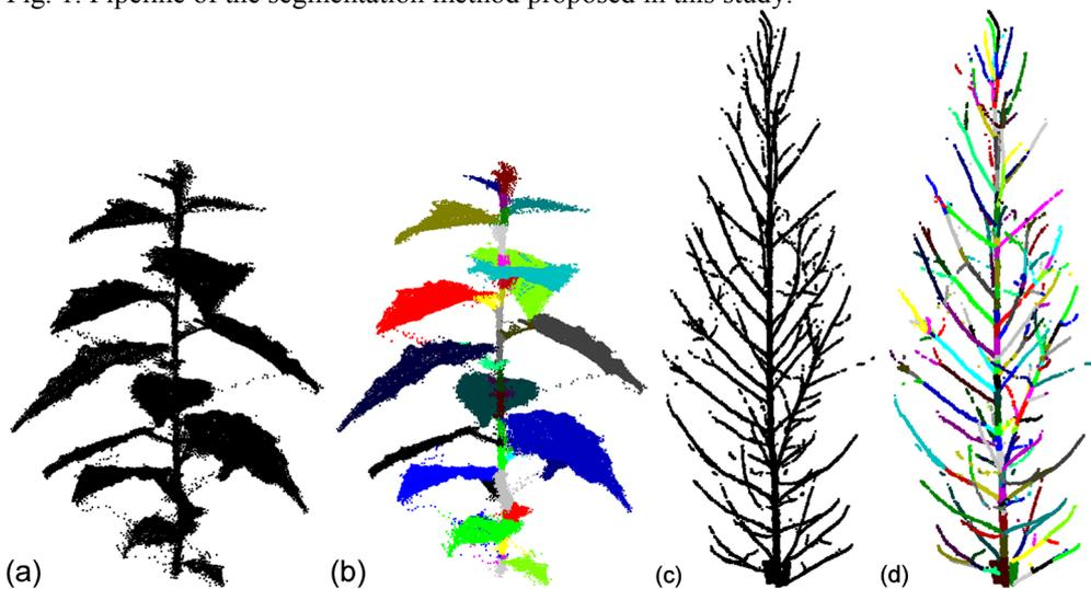
Fig. 2. Comparison of raw (a, c) and segmented (b, d) point clouds for a 0.4 m height poplar seedling (a, b) and a 3.7 m height eucalyptus tree.
