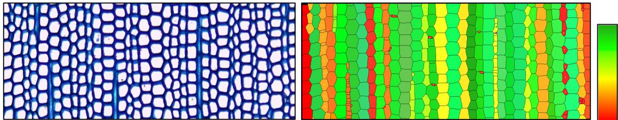
Fig. 1. Left: cross-section of *Abies alba*. Right: automated identification of radial files. Color value qualifies the reliability coefficient: weakly reliable files appear in red tones and highly reliable files are in green tones.
